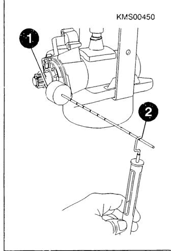
Checking armature braking torque
